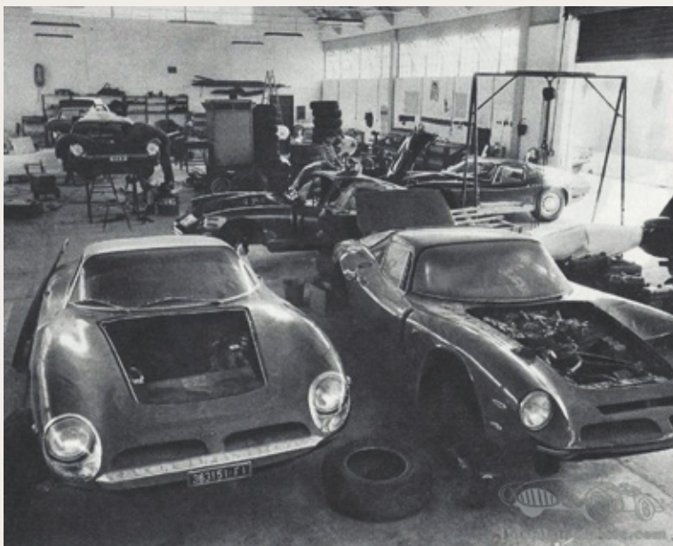
#0266 and #0242 in the factory, summer 1967, after the Mugello race as the third bonnet slit is on the car by now. Webers carburettors can be clearly seen on 0242 © DR
